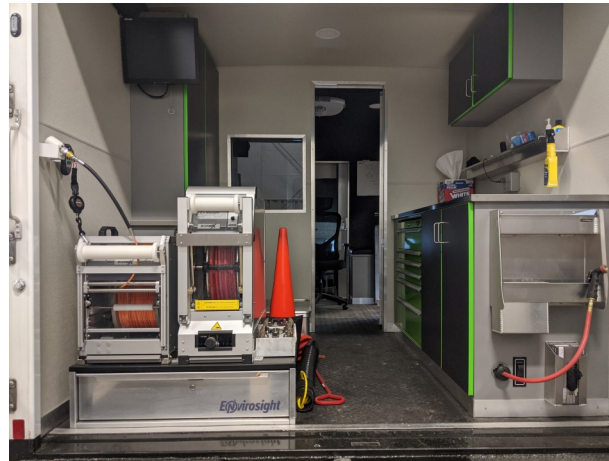
Sewer Inspection Camera Truck
