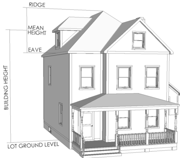
Figure 12-2: Building Height – Gable Roof
