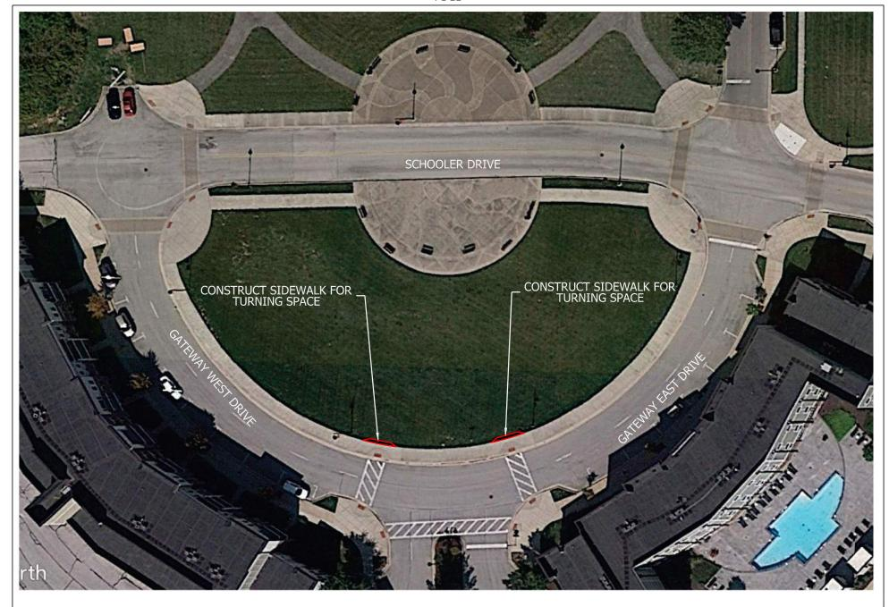
1. All Proposed lines are an approximate detail of the curb ramp. Contractor is responsible to build curb ramps per ADA Standards.
