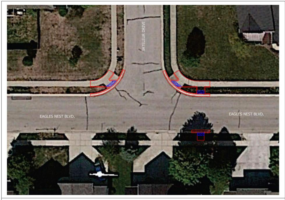
1. All Proposed lines are an approximate detail of the curb ramp. Contractor is responsible to build curb ramps per ADA Standards.
