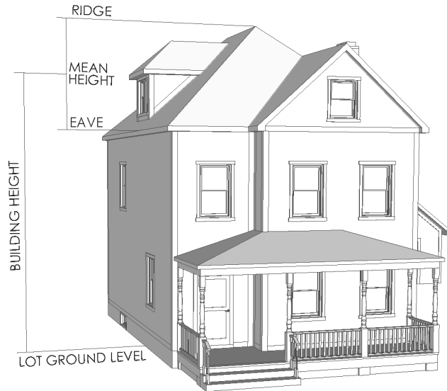
Figure 12-2: Building Height – Gable Roof
