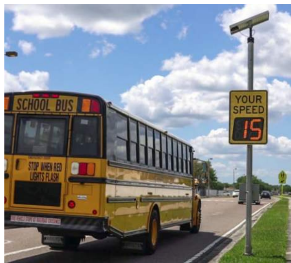
Radar speed feedback sign installed on separate post
