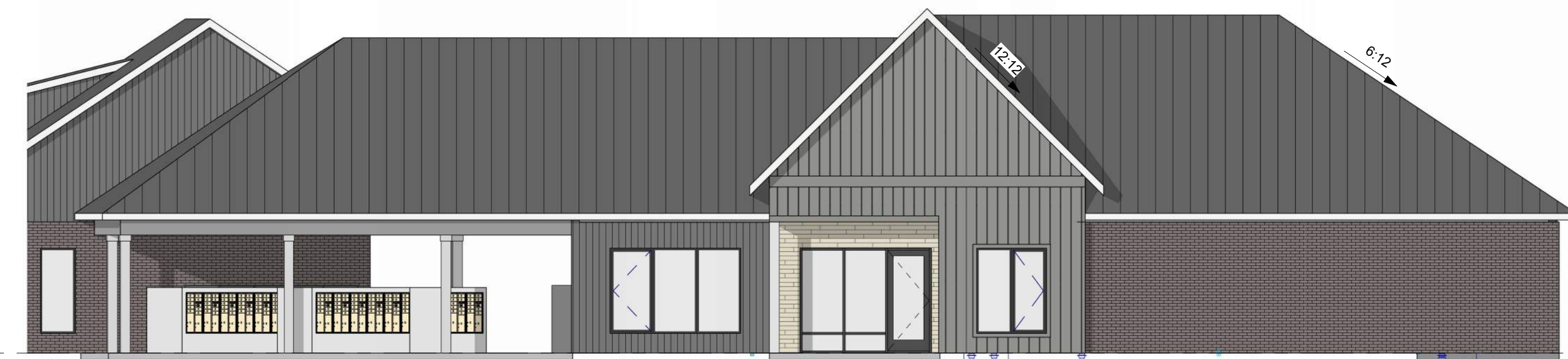
1 CLUBHOUSE - FITNESS - EAST GRAPHIC 1/8" = 1'-0" Masonry : 549 SF Non Masonry: 175 SF Doors and Windows: 197 SF Total: 724 SF Percent Masonry: 76%
