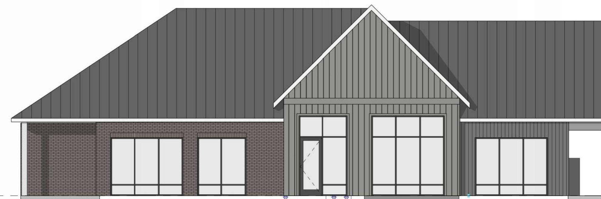
4 CLUBHOUSE - FITNESS - WEST GRAPHIC 1/8" = 1'-0" Masonry : 225 SF Non Masonry: 145 SF Doors and Windows: 401 SF Total: 370 SF Percent Masonry: 60%
