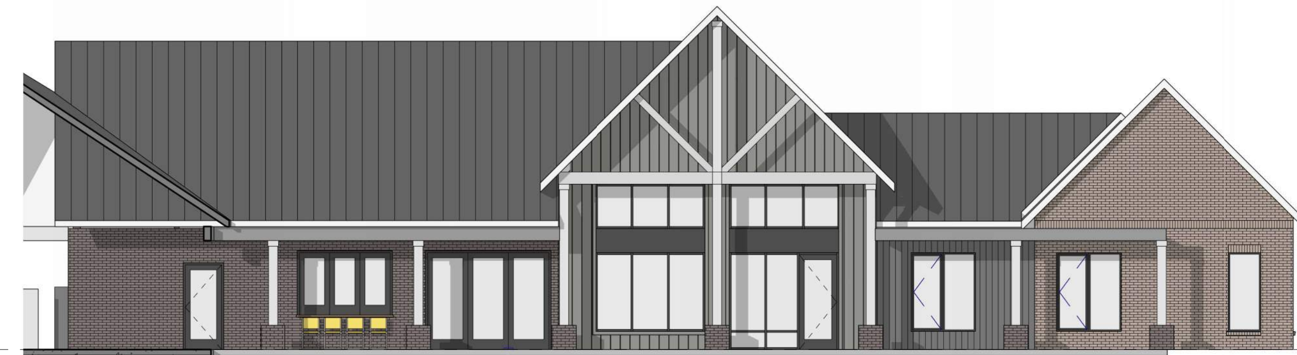
3 CLUBHOUSE - LEASING - NORTH GRAPHIC 1/8" = 1'-0" Masonry : 439 SF Non Masonry: 216 SF Doors and Windows: 430 SF Total: 655 SF Percent Masonry: 67%
