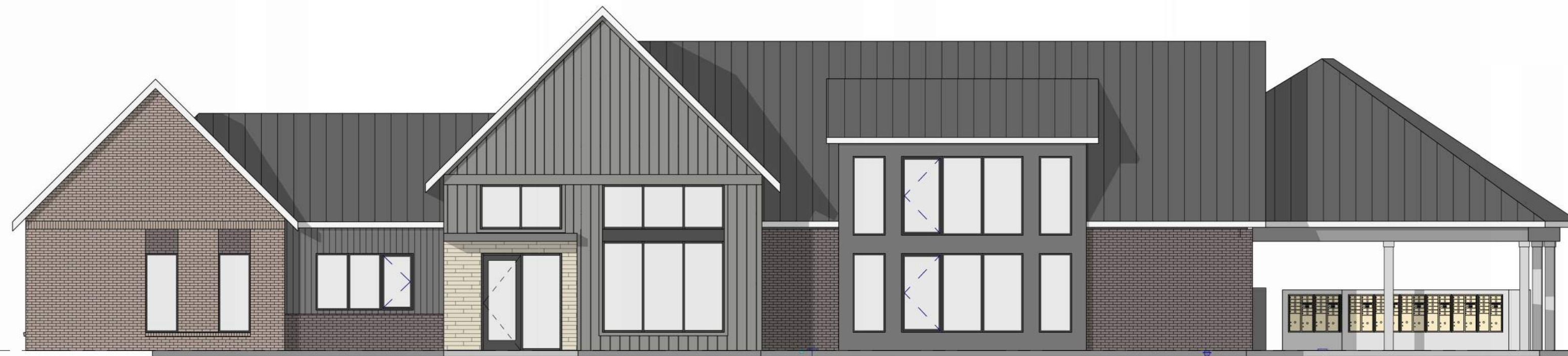
2 CLUBHOUSE - LEASING - SOUTH GRAPHIC 1/8" = 1'-0" Masonry : 420 SF Non Masonry: 289 SF Doors and Windows: 461 SF Total: 709 SF Percent Masonry: 59%
