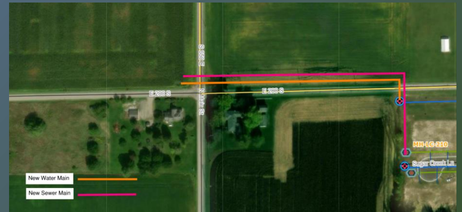
CR E 200 S Water Main Extension
