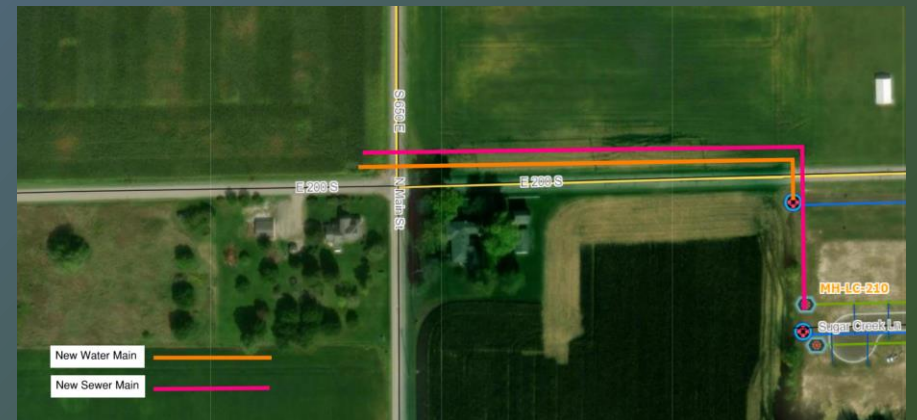
CR E 200 S Water Main Extension
